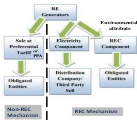
Figure: Block Diagram of REC Concept (S.K. Soonee and etal, n.d.)
