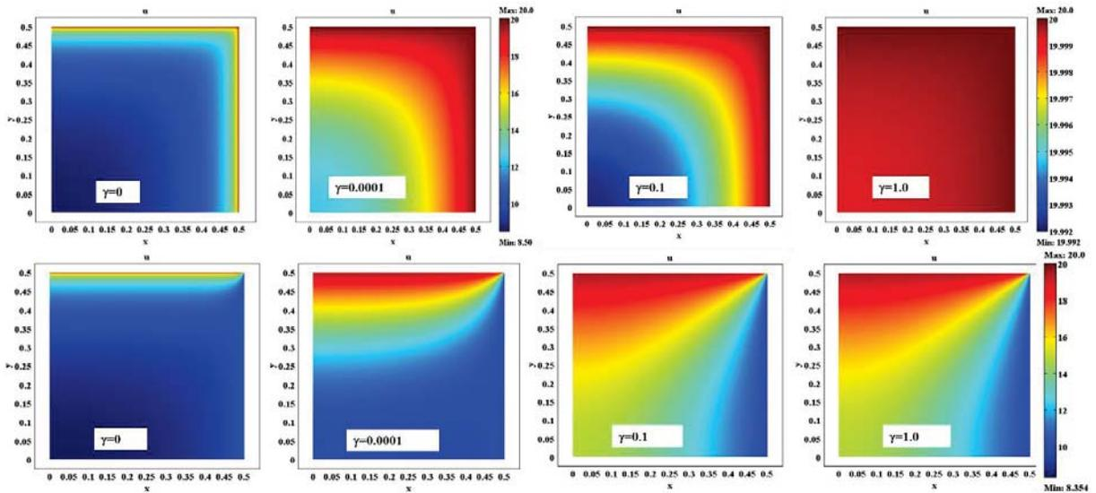
FIGURE 3. The electric potential distribution in one fourth of the cross-section for Case- I and II.
