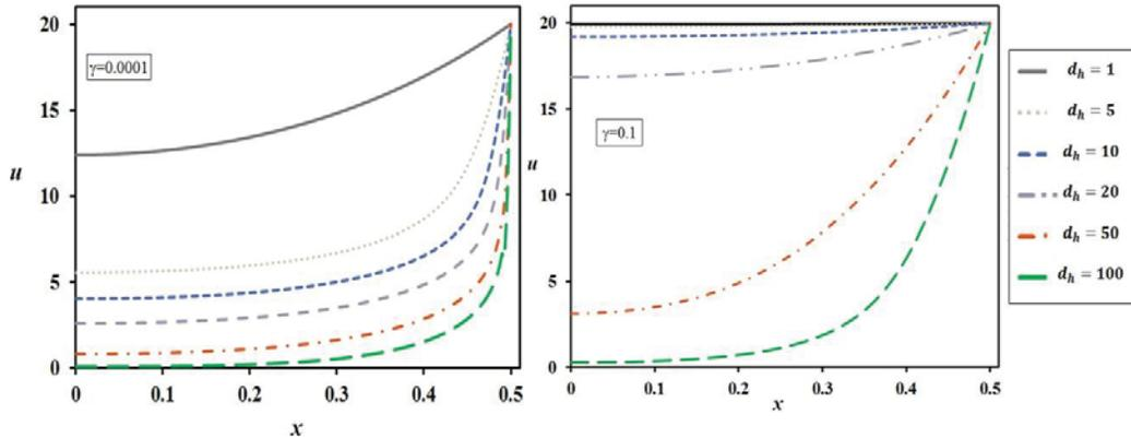
FIGURE 6. Effect of hydraulic diameter on electric potential distribution for (a)  $\gamma = 0.0001$  and (b)  $\gamma = 0.1$ .
