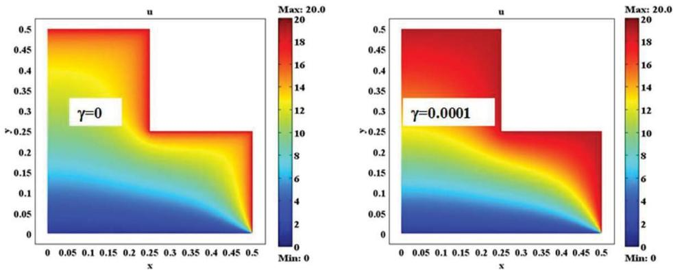
FIGURE 7. Electric potential distribution for (a)  $\gamma = 0.0$  and (b)  $\gamma = 0.0001$  for irregular geometry.
