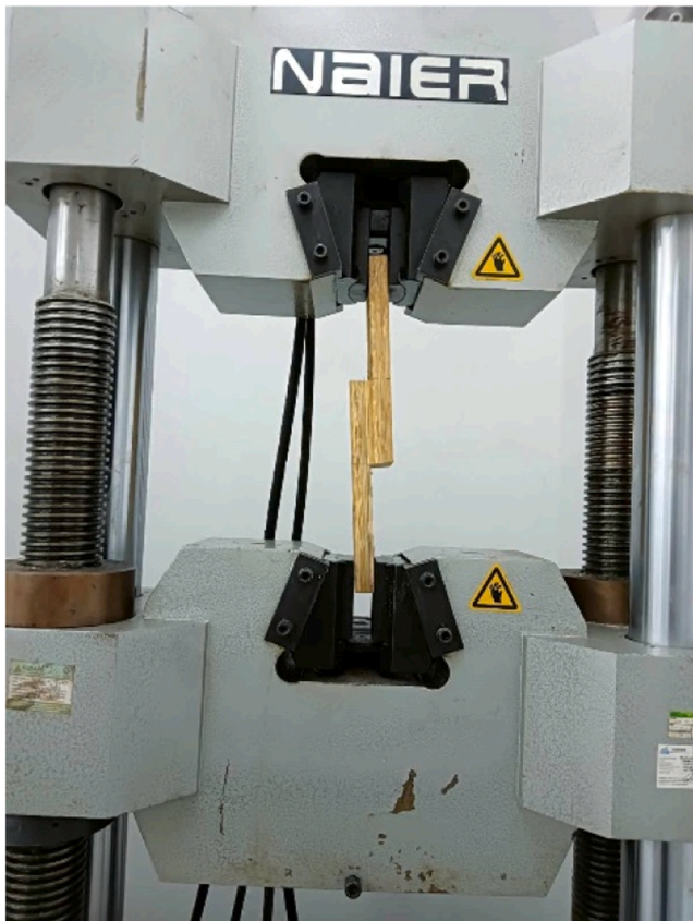
Fig. 7. Shear strength test for LBL specimen.
