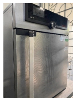
Oven-drying of laminated bamboo
