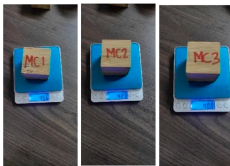
Weighing of laminated bamboo
